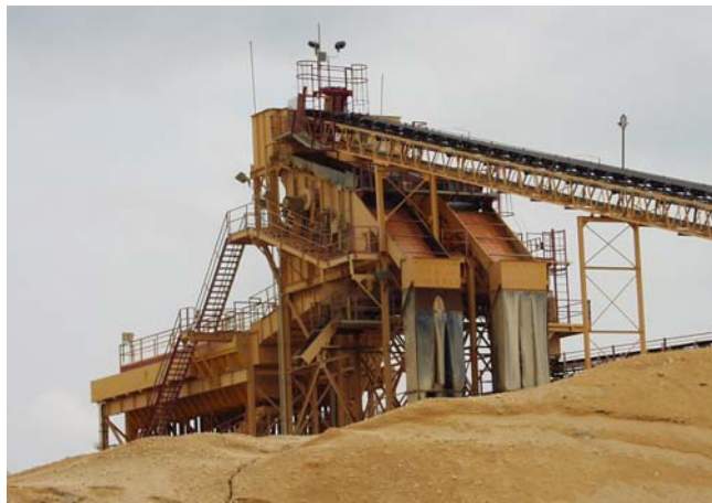
Figure 17. Diester 6- x 20-ft shaker screens.
