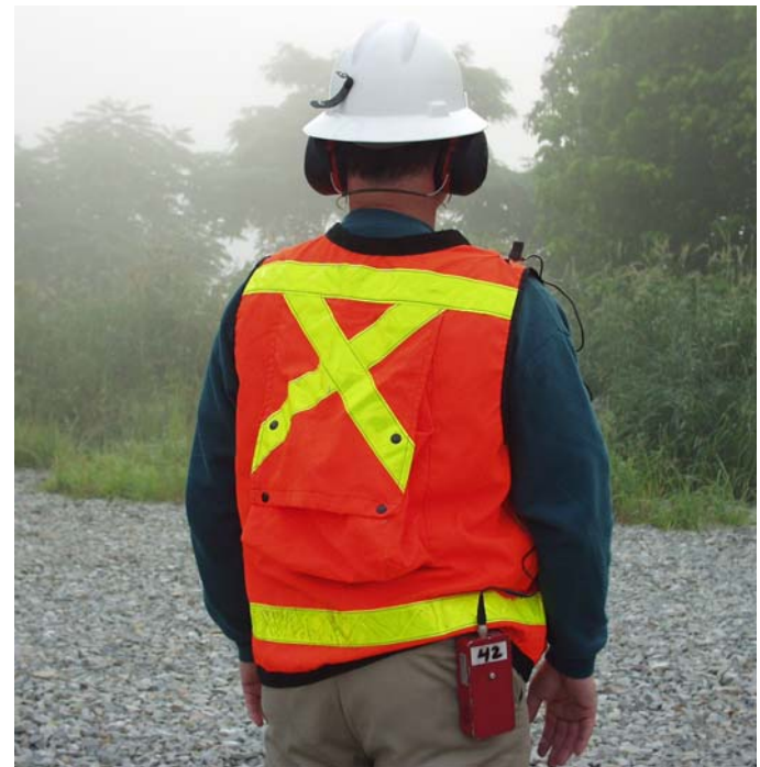
Figure 3. Noise exposure monitoring with a personal dosimeter.
