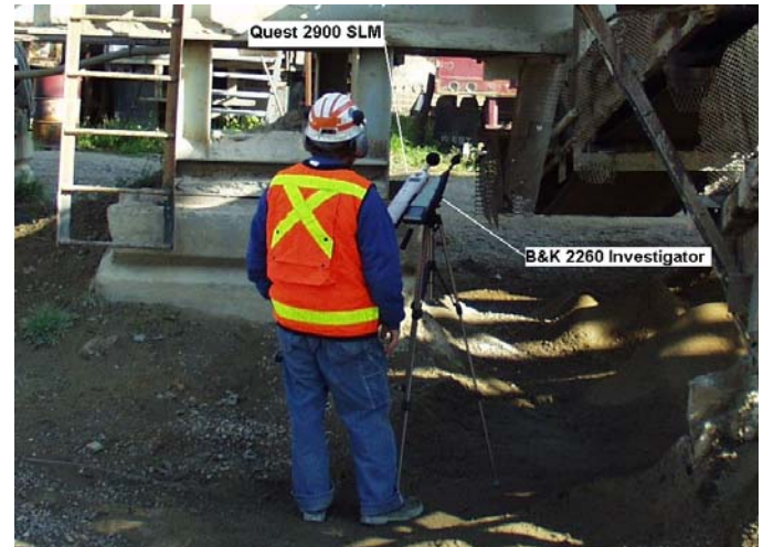
Figure 2. Sound level meters used to measure equipment noise levels.
