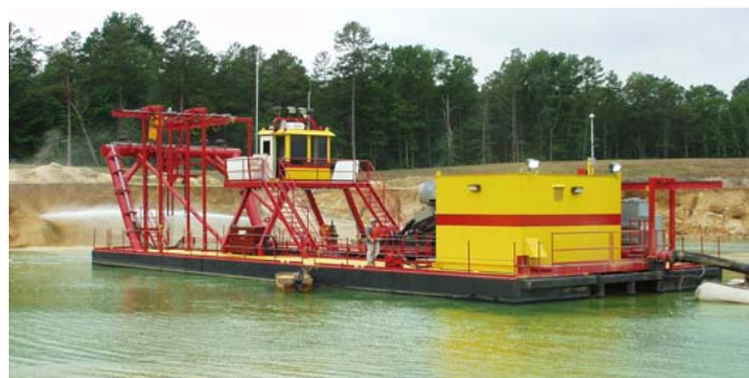
Figure 9. Electric hydraulic cutter head mining dredge.
