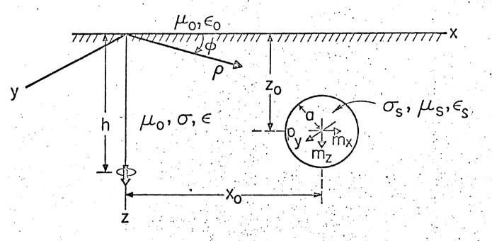
FIGURE 1. Geometry for source loop and buried sphere with induced dipole moments.
