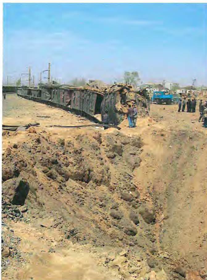
Figure 2. Crater produced by train explosion in Ryongchon, North Korea. Accident may have been the result of cars of AN coming into contact with electrical wires."
