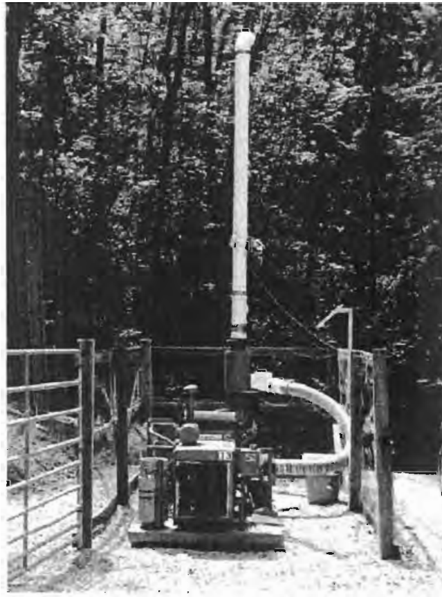
Figure 3. Instrumenting gob vent boreholes for monitoring.
