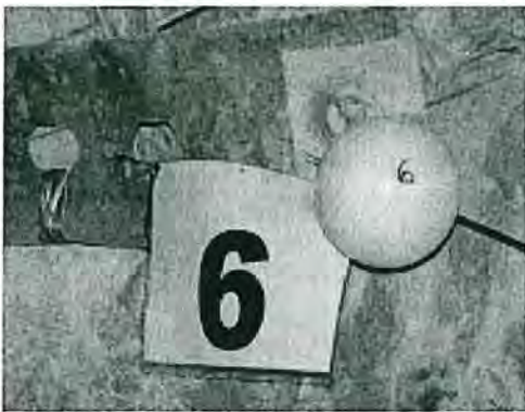
Figure 3. Example of NIOSH-developed rib-mounted spherical target and identification placard used to merge overlapping scan areas.
