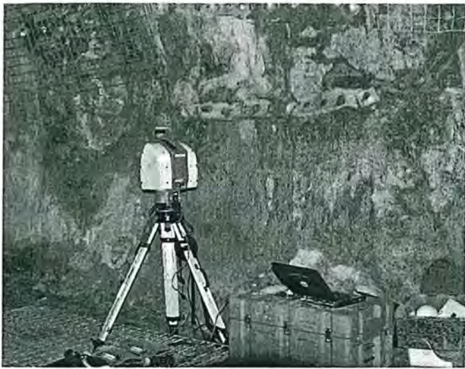
Figure 2. Typical field setup of the laser scanner and laptop computer.
