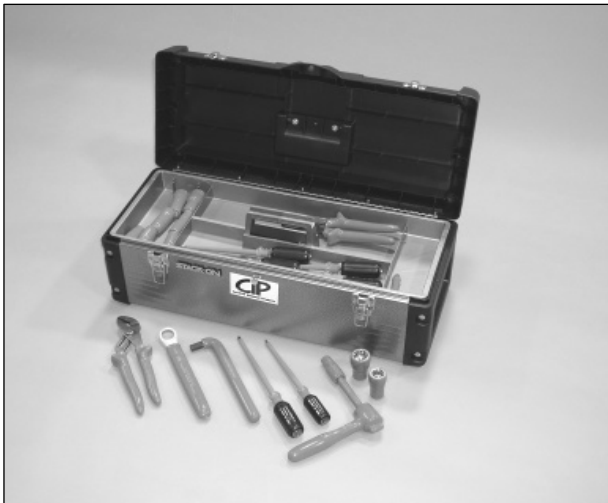
Figure 4. Hand tools electrically rated for 1000Vac can significantly reduce the likelihood of starting an electrical arc if accidentally dropped into equipment.
