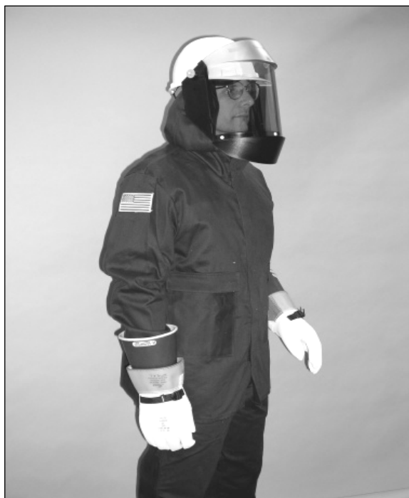
Figure 3. This worker is dressed for Hazard/Risk Category 2. He is wearing a hooded jacket and bib-overalls over FR work clothes, a combination face shield/hardhat over safety glasses, and voltage-rated gloves with leather protectors.
