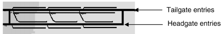
Fig. 11. An example layout showing additional horizontal, in-seam boreholes on either side of the gateroads in addition to pattern A. The entries represent a three-entry system with intervening coal pillars.
