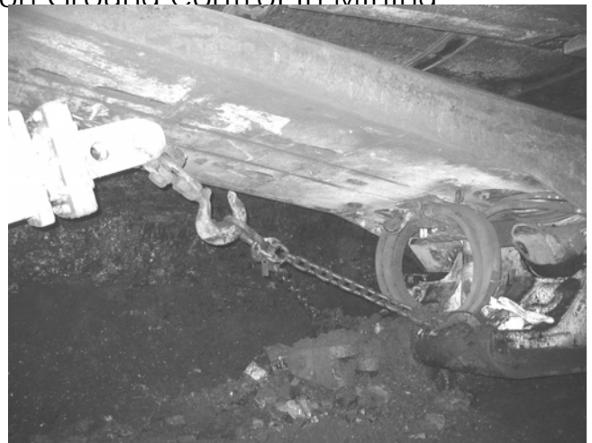
Figure 4. Shield retriever advancing walking shield.
