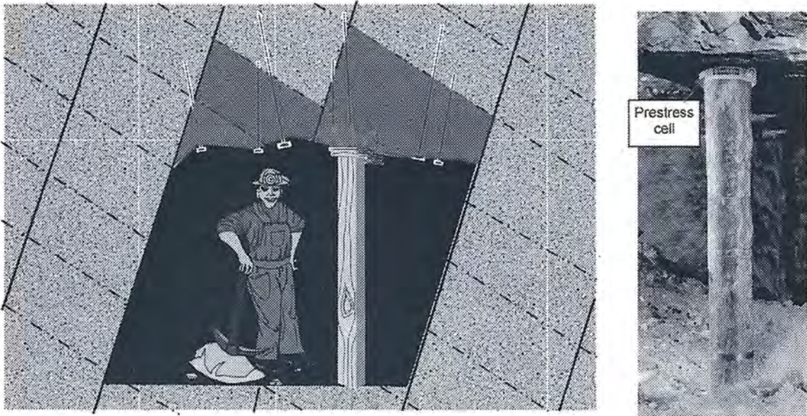
Figure 5: Water inflatable prestressing bladder used to preload a timber post and provide active roof loading to a traditionally passive support.
