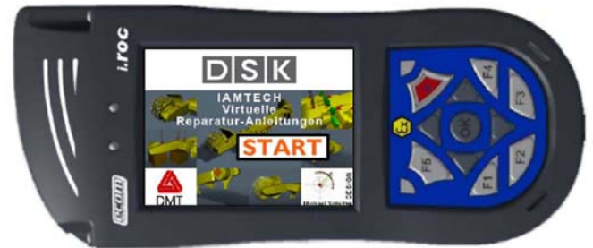
Figure 4. Repair assistance on PDA
