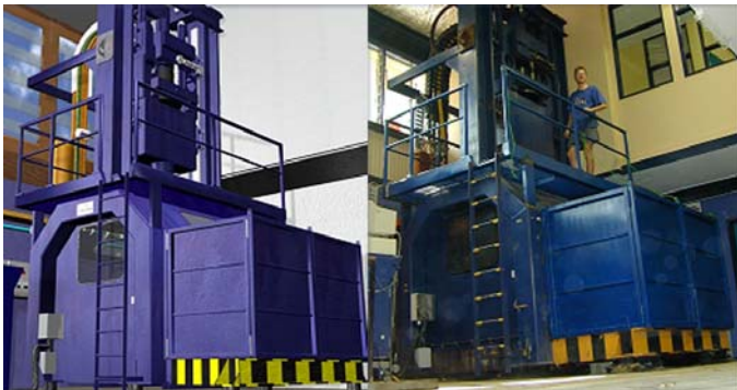
Figure 2. Left - simulated drill rig, Right - actual drill rig
