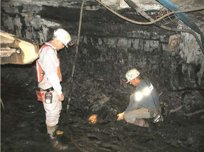
Figure 4. Two workers completing a dual lift when hanging cable.
