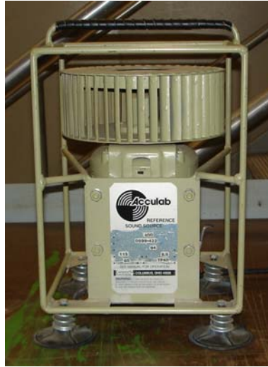
Figure 3: Calibrated Noise Source for Underground Testing
