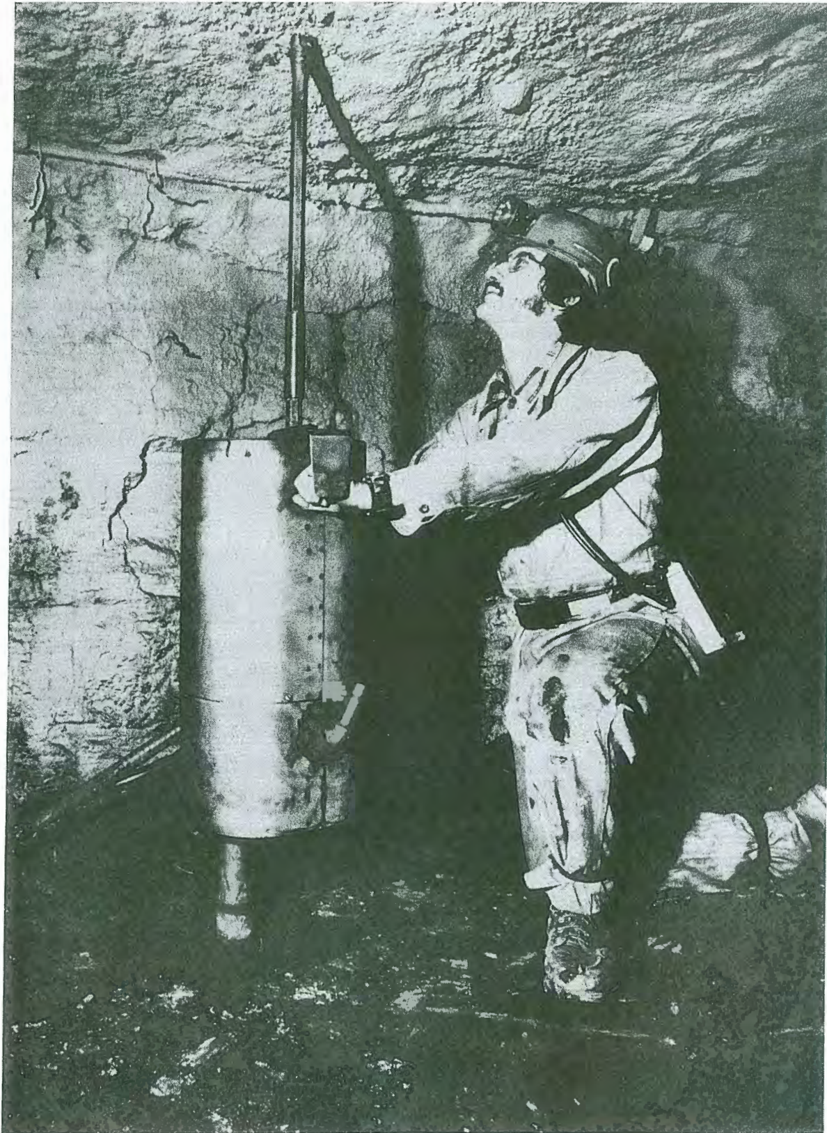
FIGURE 5. Pneumatic drill noise control system that reduces levels to approximately 95 dbA.
