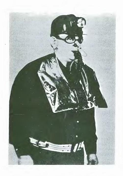
FIGURE 5. Ten-minute self-rescuer developed under a Bureau research contract by the Mine Safety Appliances Company (Bureau of Mines, U. S. Department of the Interior).
