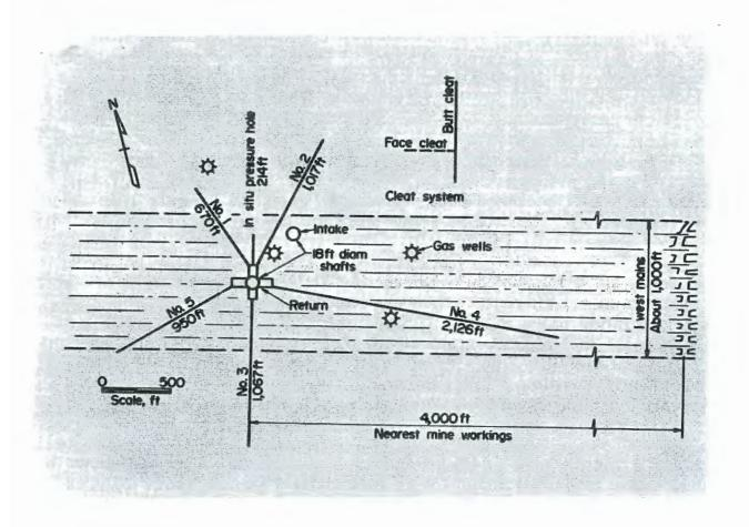
FIGURE 11. Ventilation shaft of the Pittsburgh seam of Eastern Associated Coal Corporation for draining methane in advance of mining (Bureau of Mines, U. S. Department of the Interior).
