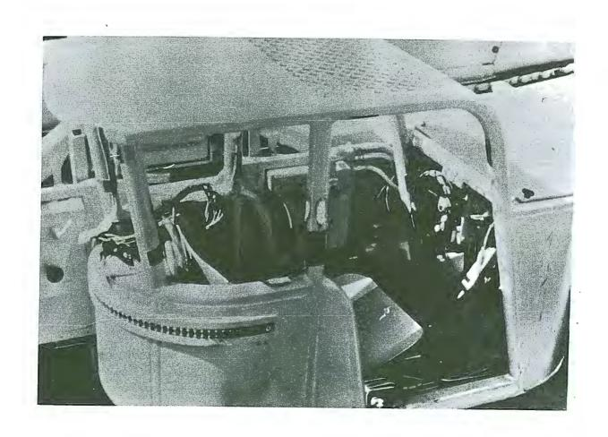
FIGURE 14. Human-engineered cab for four-foot seam face use (Bureau of Mines, U. S. Department of the Interior).
