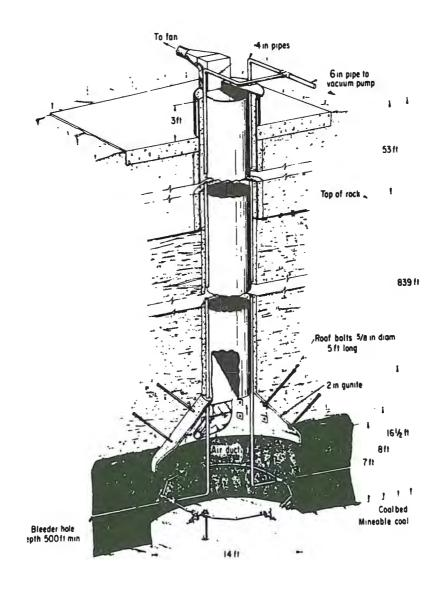
FIGURE 10. Multipurpose borehole for degasification of virgin coal (Bureau of Mines, U. S. Department of the Interior).
