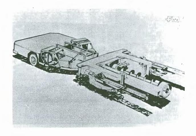
FIGURE 13. Auger cutter with face drills (Bureau of Mines, U. S. Department of the Interior).
