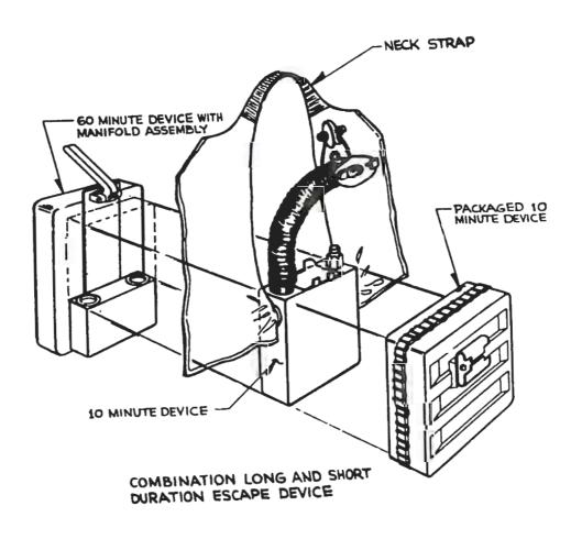
FIGURE 7. A self-rescuer with an initial canaster developed under a Bureau research contract with the Mine Safety Appliances Company (Bureau of Mines, U.S. Department of the Interior).
