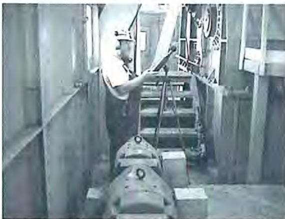
Figure 2 — Example of noise measurement at a worker location.
