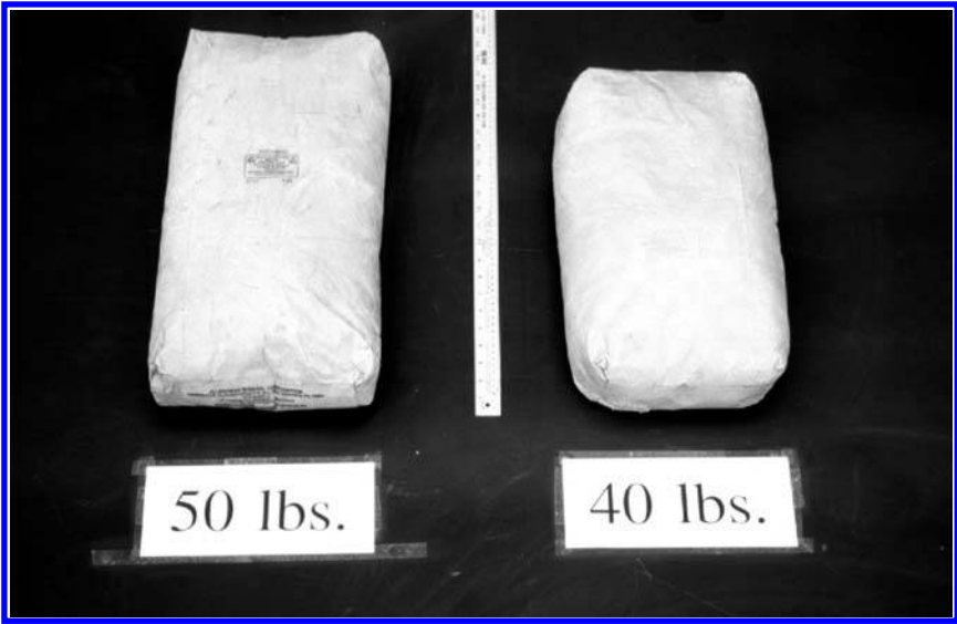
FIGURE 43.6 Redesign of a standard 50-lb (23 kg) bag to 40 lb (18 kg) was achieved by working with supplier, and creates a more acceptable load for workers operating in restricted postures.
