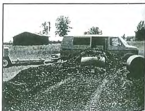
Figure 6.—First layer of coal covering electrode grid and first perforated plastic barrel being covered horizontally on coal pile.
