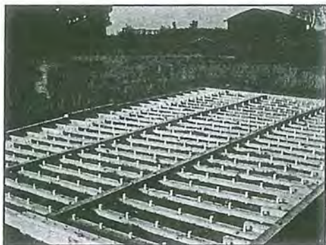
Figure 3.—Completed wood frame with PVC pipe holders.
