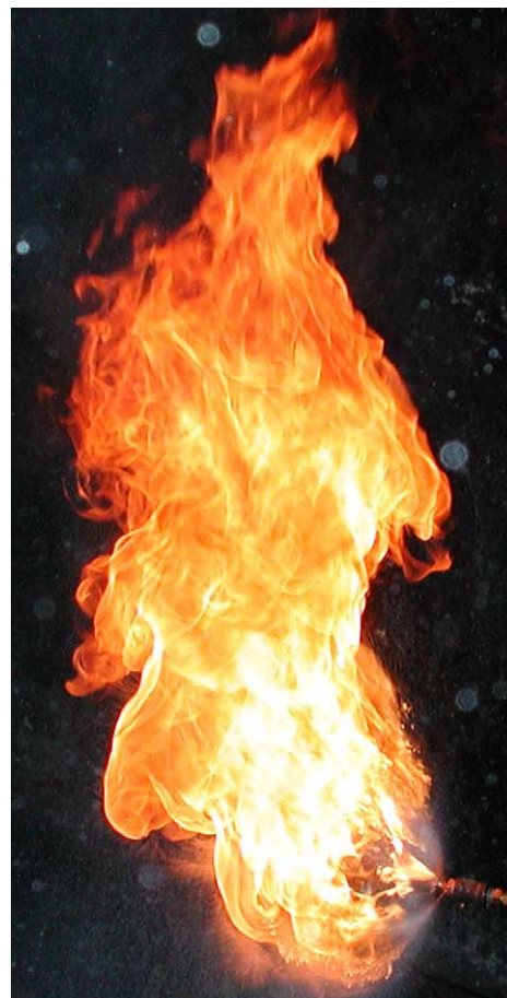
Fig. 2. A typical hydraulic oil spray flame.
