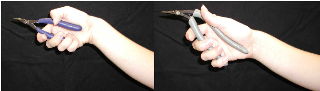
Figure 1.1: Sagittal view of straight-handle pliers (left) and bent-handle pliers (right).
