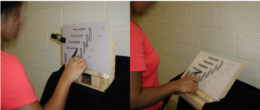
Figure 3.6: Vertical (left) and 45° slanted (right) work surface orientations used in experiment.
