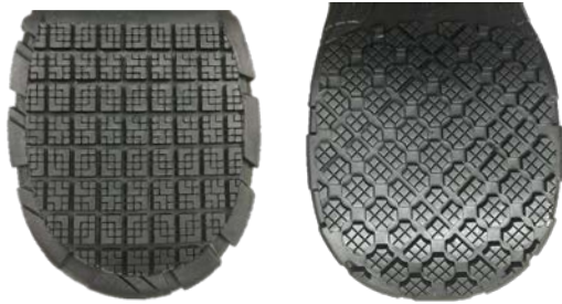
Figure 1. Tread designs of two shoe types. Shoe A (left) had a sharp-edged heel with rectangular tread and Shoe B (right) had a beveled heel with diamond shaped tread.
