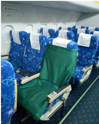
Fig. 2. Photo of the pressure mats positioned on the seat.
