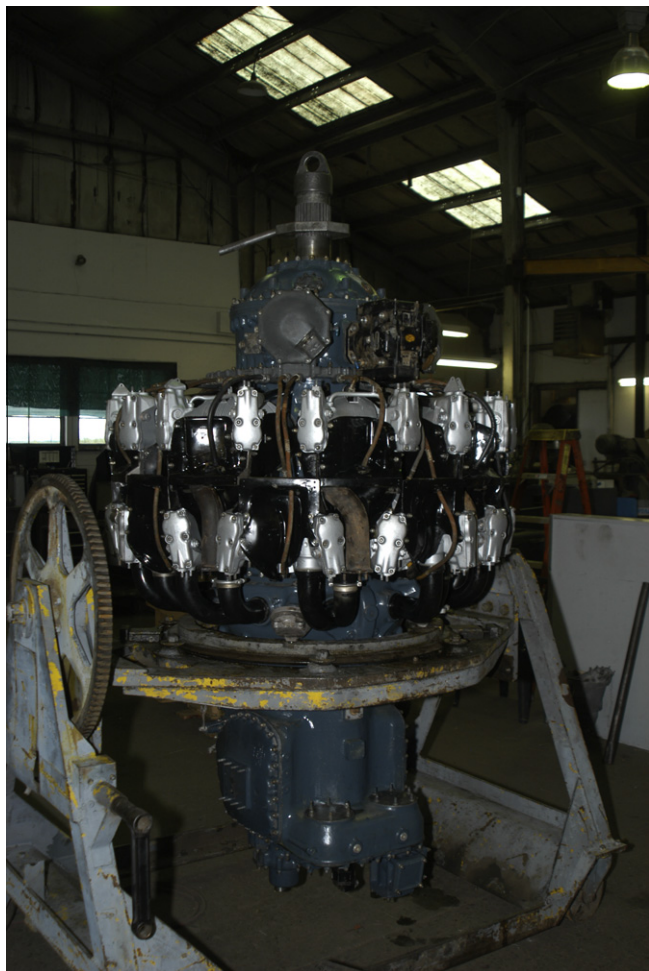
Fig. 1. Pratt & Whitney R2800-30W engine used in the present study. The engine is pictured at the completion of the study supported in a maintenance frame.
