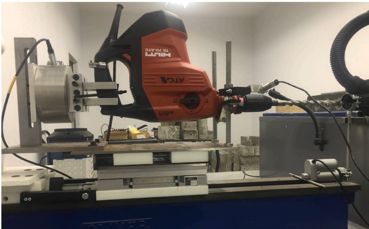
Fig. 1. Experimental setup. Drill handle is attached to 6-axis load cell with finger-like clamps. The platform supporting the drill and load cell slides on a lathe bed and is advanced by a linear actuator. A hose clamp on the handle secures the accelerometer to the handle. During drilling, the drill bit moves through a vacuum attachment into a block.
