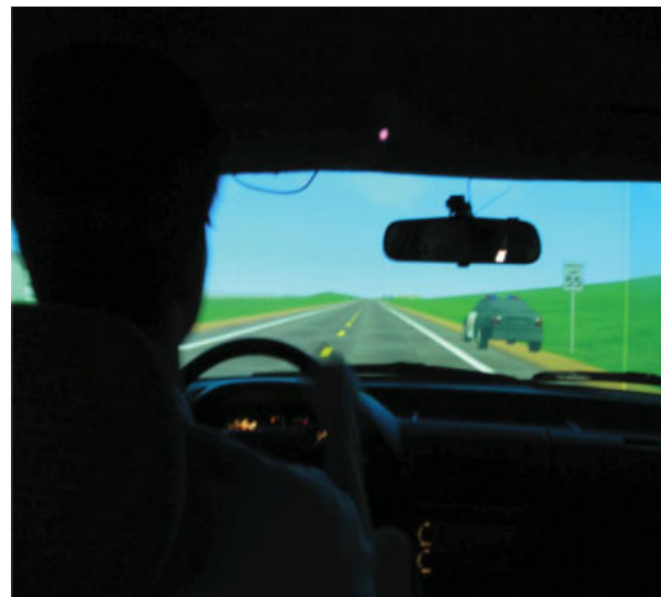
FIG. 1. A: An “over the shoulder” view shows setup of a driver in SIREN approaching the police car parked by the side of the virtual road. B: Normal response: A driver slows down and moves to the left. [Color figure can be viewed in the online issue, which is available at www.interscience.wiley.com .]
