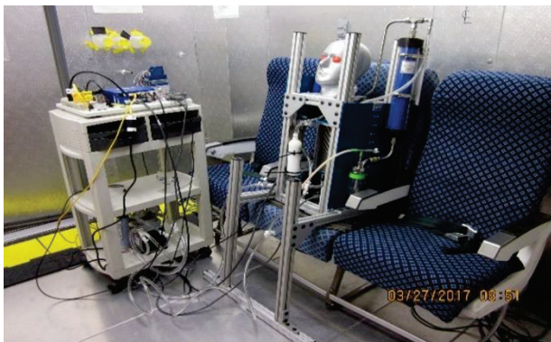
Figure 3 Utilized coughing manikin. Adopted from (Noti et al. 2017)
