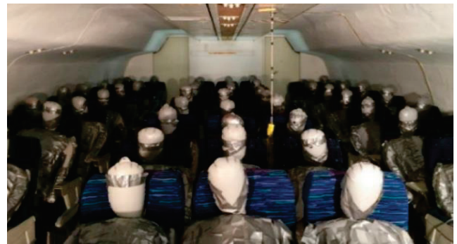
Figure 2 Boeing 767 cabin mock-up with heated manikins
