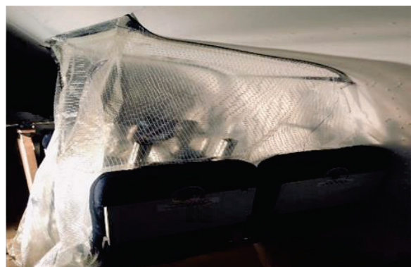
Figure 4 The coughing manikin inside the ISOPass
