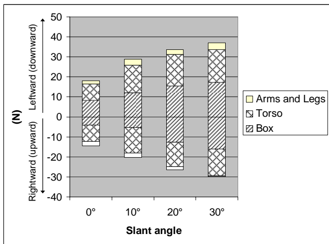
Figure 5. Overall and component analysis of peak lateral forces as a function of lateral slant angle.
