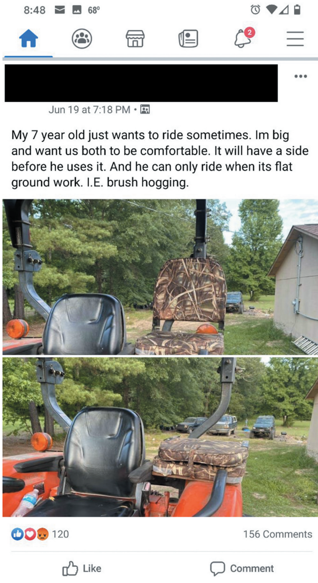
Figure 1. Homemade child seat attached to tractor fender.
