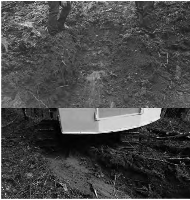
Figure 6. Top: shear plane resulting from sliding of an untethered harvester on wet clay soils. Bottom: stabilized machine after sliding was arrested.
