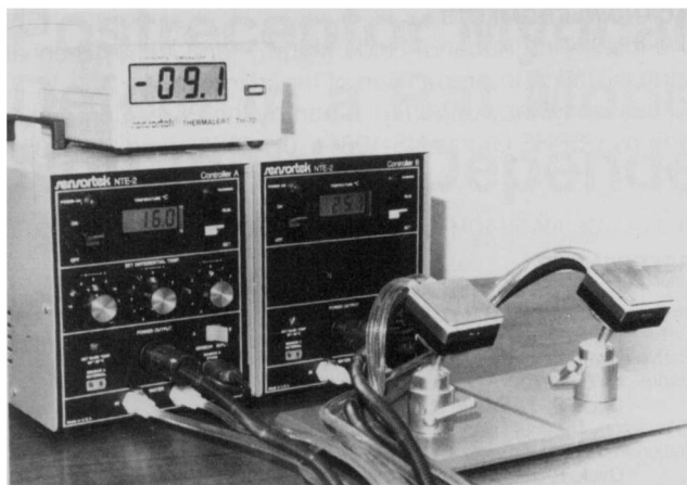
FIGURE 1. The Thermal Sensitivity Tester, including two digitally controlled power units, two standard plates, and a differential thermometer. The water pumping unit is not shown.
