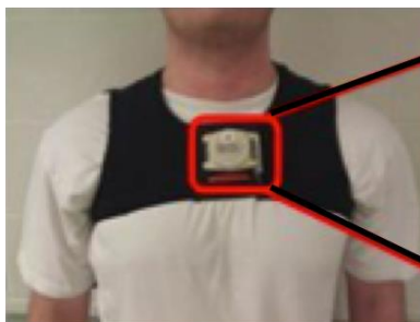
Figure 2: Attachment of IMU sensors at sternum level using Velcro strap.
