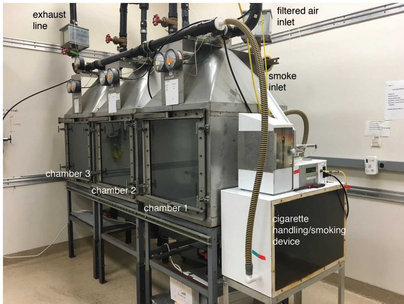
Figure 1. Tobacco smoke exposure chambers. From right to left, in chambers 1 to 3, the averaged chamber total suspended particulate (TSP) concentrations for the entire exposure period were 87 \text{ mg/m}^3 , 57 \text{ mg/m}^3 , and 44 \text{ mg/m}^3 , respectively. The average TSP concentration over the 39-week exposure period was approximately 63 \text{ mg/m}^3 .
