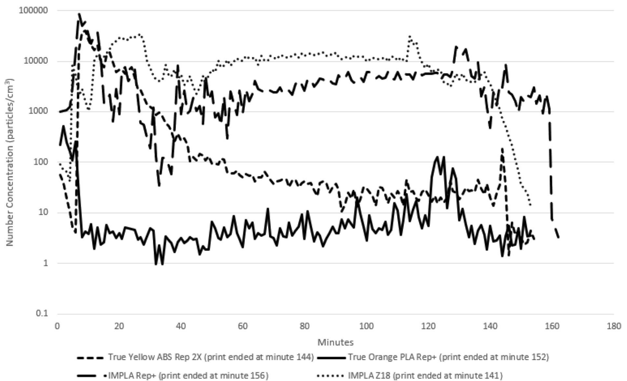
Fig. 5 Total number concentration of ultrafine particles from 10 to 420 nm from chamber tests with individual printer and filament combinations
