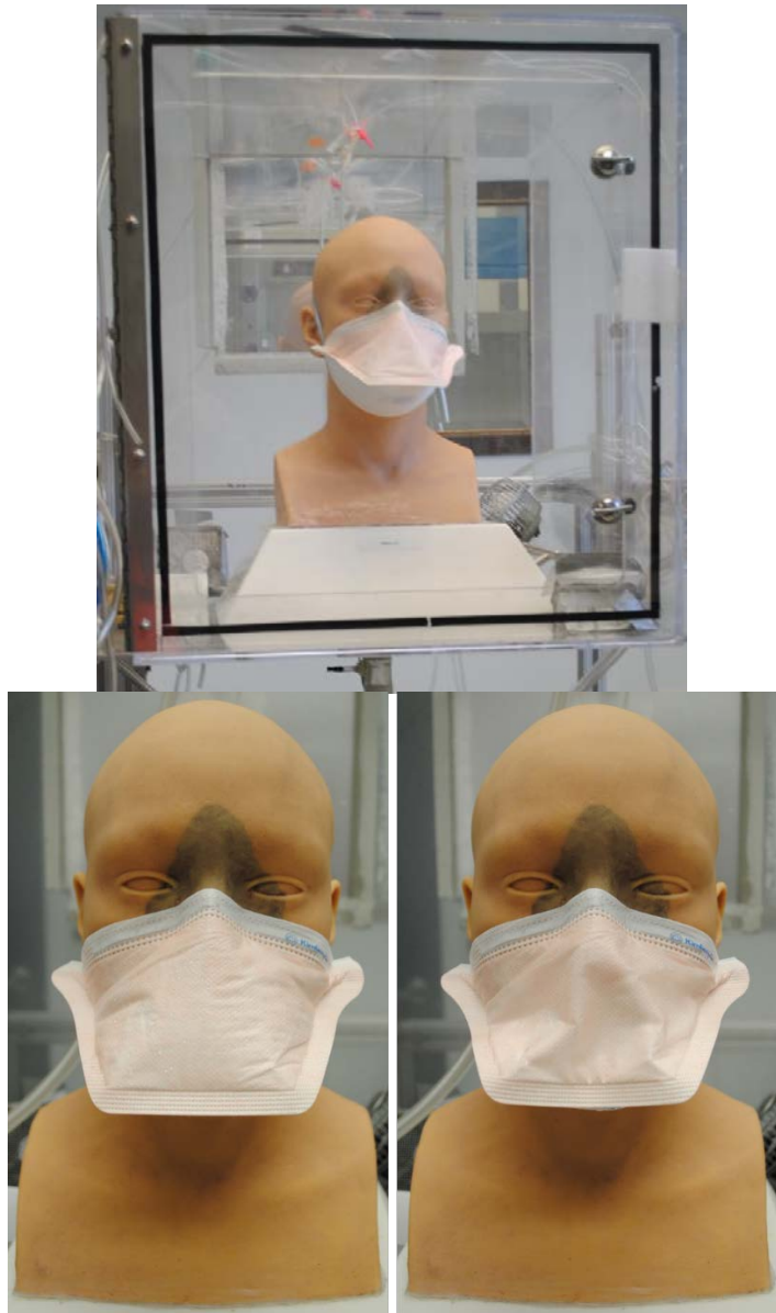
Figure 1a. A flat fold respirator (Kimberly Clark 46727) mounted on a headform at no breathing condition inside the test chamber (Top).
