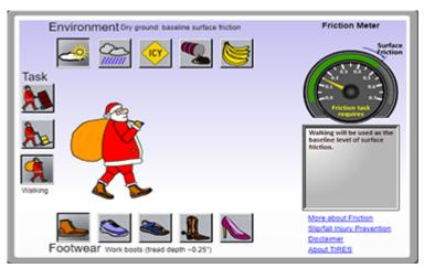
Slips, trips and falls are a major cause of injuries in the trucking industry. The correct amount of friction prevents these injuries. Friction can be measured using the 'Coefficient of Friction (CoF)', which is proportional to grip between your shoes and walking surface. Friction changes with environment and contaminants, type of shoes and task activities.
