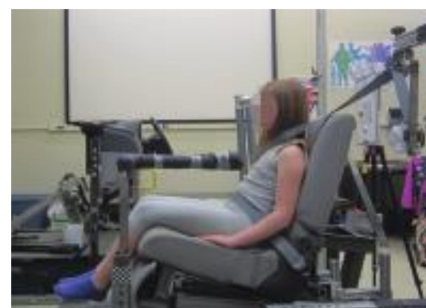
Mockup C: Cushion Length: 523 mm. D-ring re Hpt: {474, 244, 588}. XZ angle: 39 deg.
