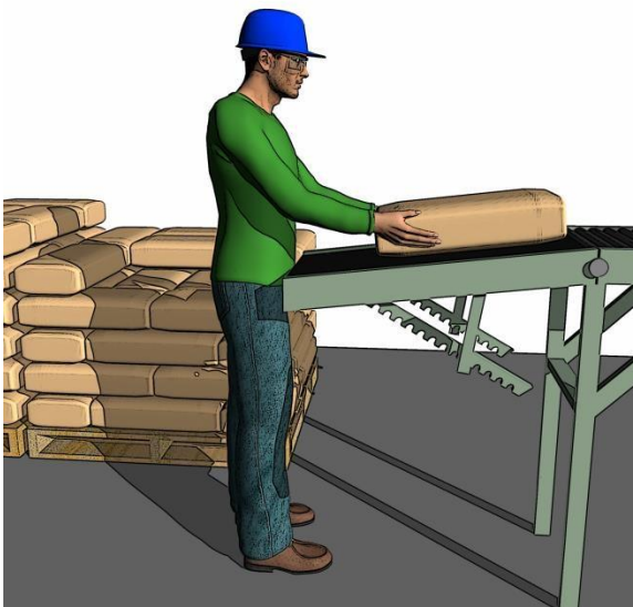
Figure A45. Worker standing at conveyor belt with an adjustable tilt end.
