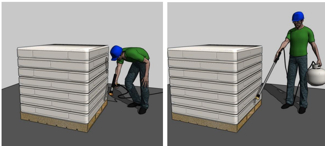
Figure A65. Short wand requires worker to bend forward to reach bottom of pallet (left). Long wand enables worker to reach bottom of pallet without bending forward (right).
