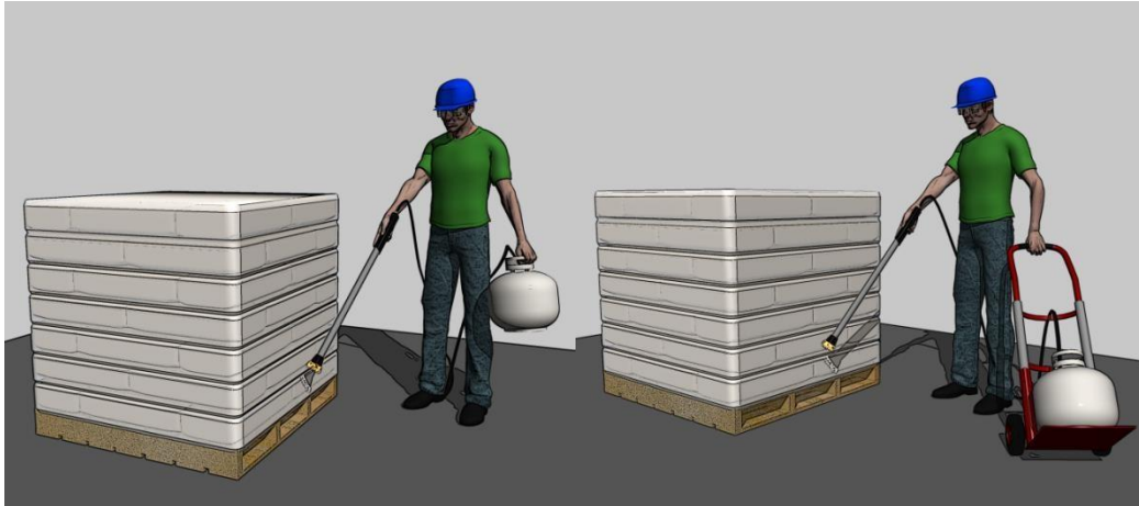
Figure A66. Worker carrying gas tank while shrink wrapping pallets (left). Manual handling is reduced by placing the gas tank on wheeled cart (right).
