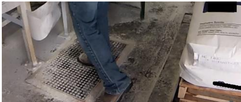
Figure 3: Anti-fatigue mat for bagger one
