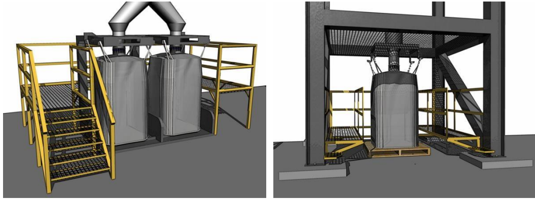
Figure A52. Platforms used to improve access to hooks and filling spout.
