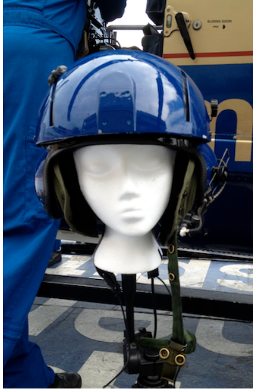
Figure 10: Testing Mannequin – Wearing Helmet
