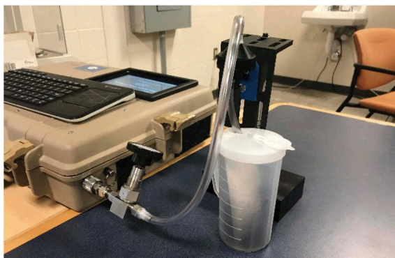
Figure 3. Experimental setup showing sampling jar attached to the AG-4000.
