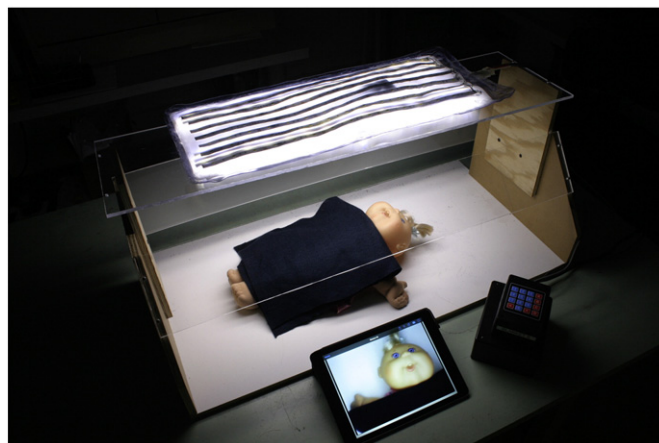
Fig. 4. The prototype Lumi-nate illumination system for incubators. The lighting system is designed to fit on top of an infant incubator and under a blanket that is often used to cover the incubator. When used as a procedural light, the Lumi-nate system provides diffuse white illumination of 2000 lux to minimize shadows. When positioned under a blanket the light is programmed to provide “cool” illumination of 600 lux during the morning and “warm” illumination of 6 lux at night to promote circadian entrainment for the infant. The Lumi-nate system always provides flicker-free illumination of excellent color rendering. The Wi-Fi enabled camera imaging system can display remotely on a tablet.
