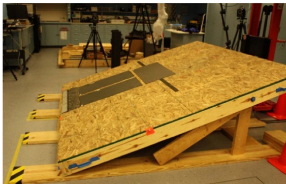
Fig. 5. Wooden platform for roofing simulation.
