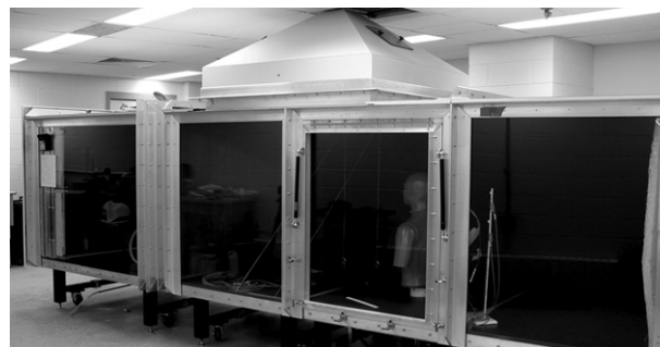
Fig. 2 Photograph of the ultralow-speed wind tunnel.
