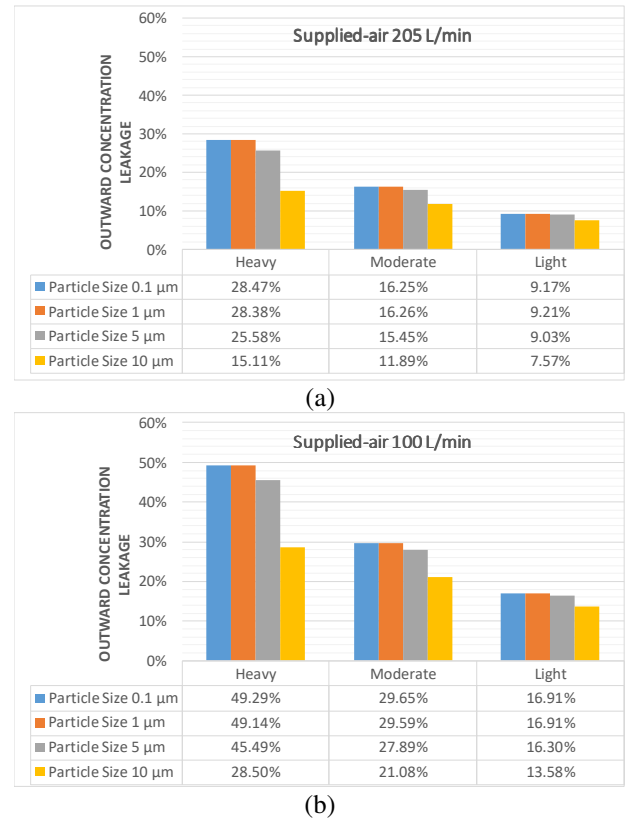
Figure 5: Concentration outward leakage of different particle sizes, breathing conditions, and supplied-air flow rates; (a) supplied-air flow rate 205 L/min, and (b) supplied-air flowrate 100 L/min.
