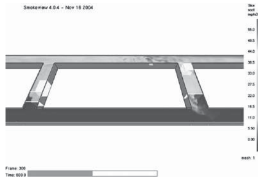
Figure 11. Smoke density distribution near the roof at 600 s for the 660 kW fire.
