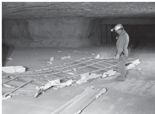
Figure 7. Debris from the X-6 steel panel stopping after LLEM test #458, looking toward B-drift.
