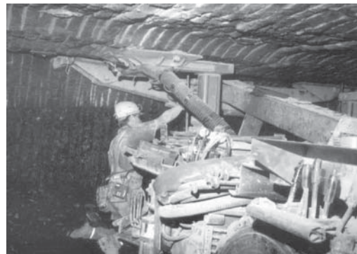
Figure 4. Canopy air curtain installed on roof bolter.
