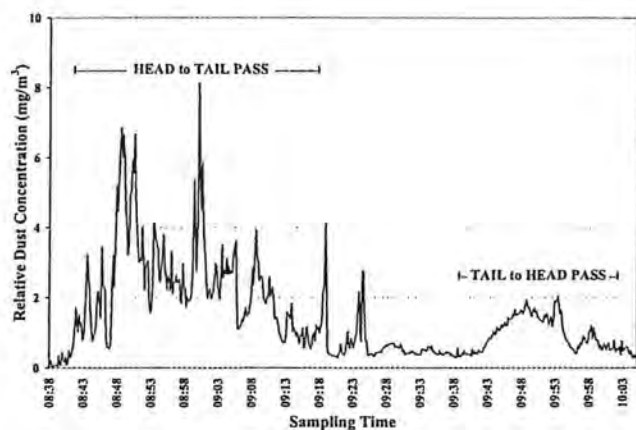
FIG 5 - Dust profile at shearer midpoint during cutting passes in each direction.
