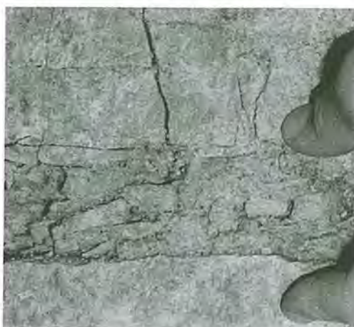
Figure 4. Disrupted zone of closely spaced mining-induced extension fractures indicating activation of zone as a flat fault.
