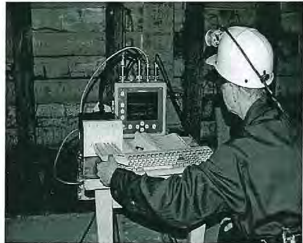
Figure 1. Engineer monitoring SIR-2 unit during a GPR survey.
