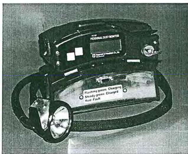
Figure 2. PDM installed on charging/communication module.
