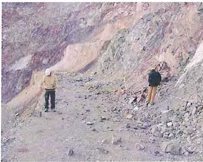
Figure 2: Students measuring the bench width and idealized cross section.
